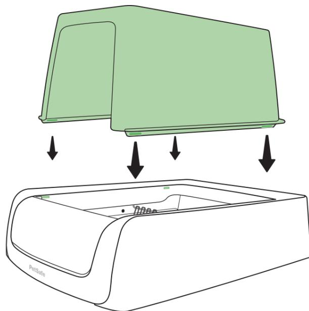
**EN** If your litter box came with a privacy cover, place it on top of the litter box, lining up the tabs at the bottom of the privacy cover with the notches in the top edge of the litter box. Press down firmly on the privacy cover to ensure all four tabs snap into place.
