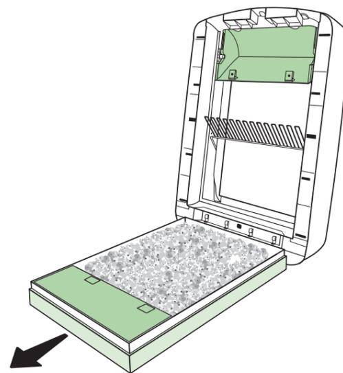
**EN** Lift the litter box frame and remove the used litter tray.
